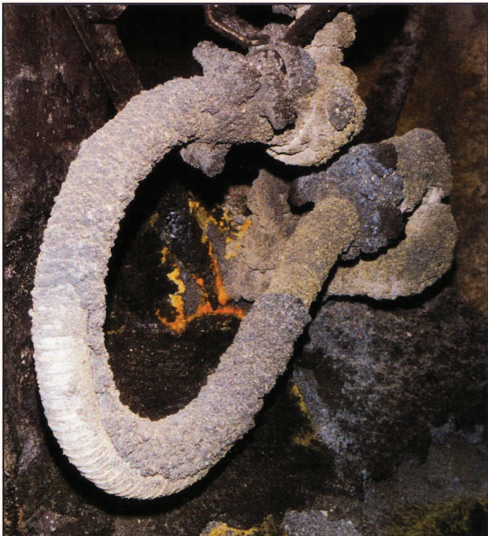
GSM Steam and Black Liquor Hose used in the Pulp and Paper industry.
