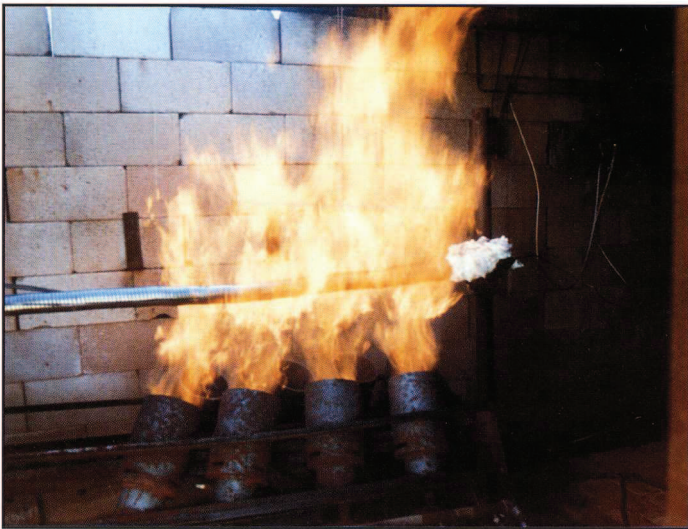
GSM BOP Hose tested at 2000°F, 2,000,000 BTU's, at 5000 PSI Working Pressure.
